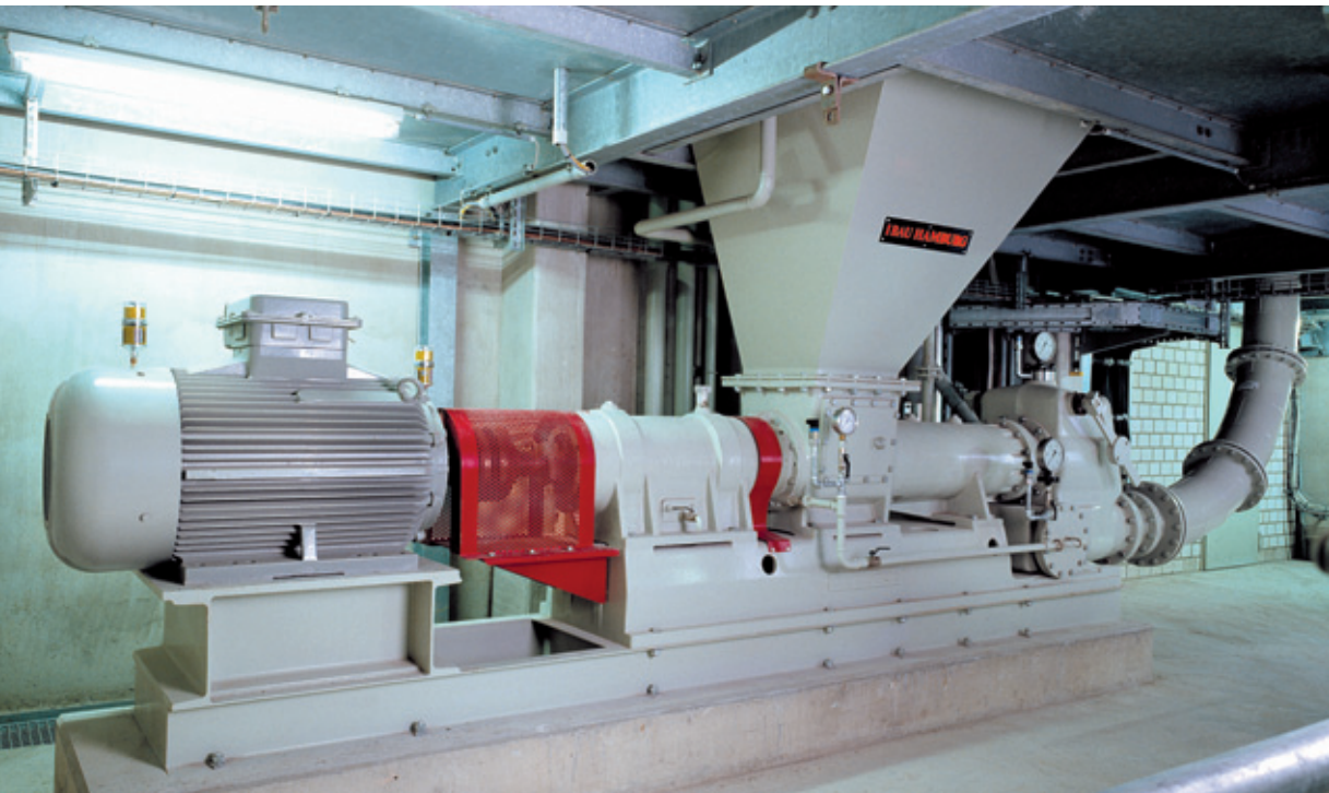
IBAU Screw pump for material transport to the preheater
