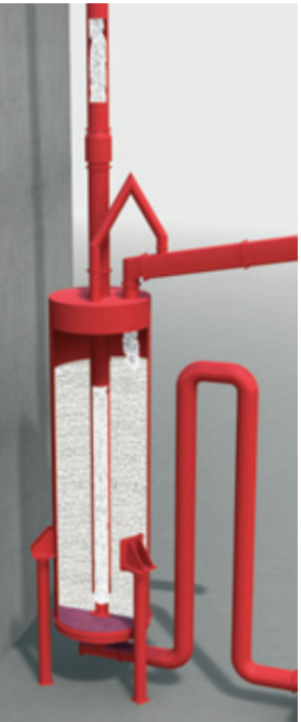
IBAU Airlift system for the material transport
