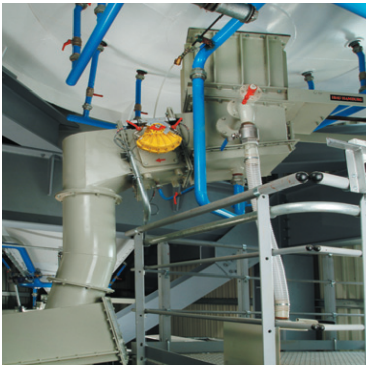
IBAU Flow control gate with pneumatic actuator and control device
