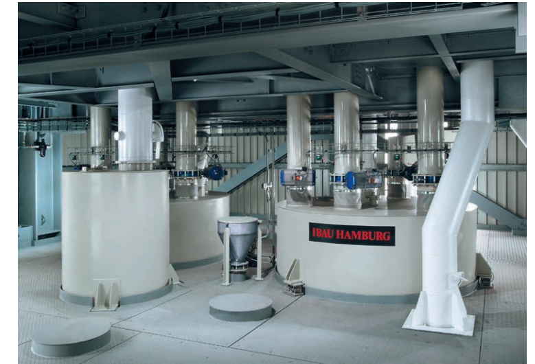
Feeding of up to 4 weighing bins for a batch-type mixing plant
