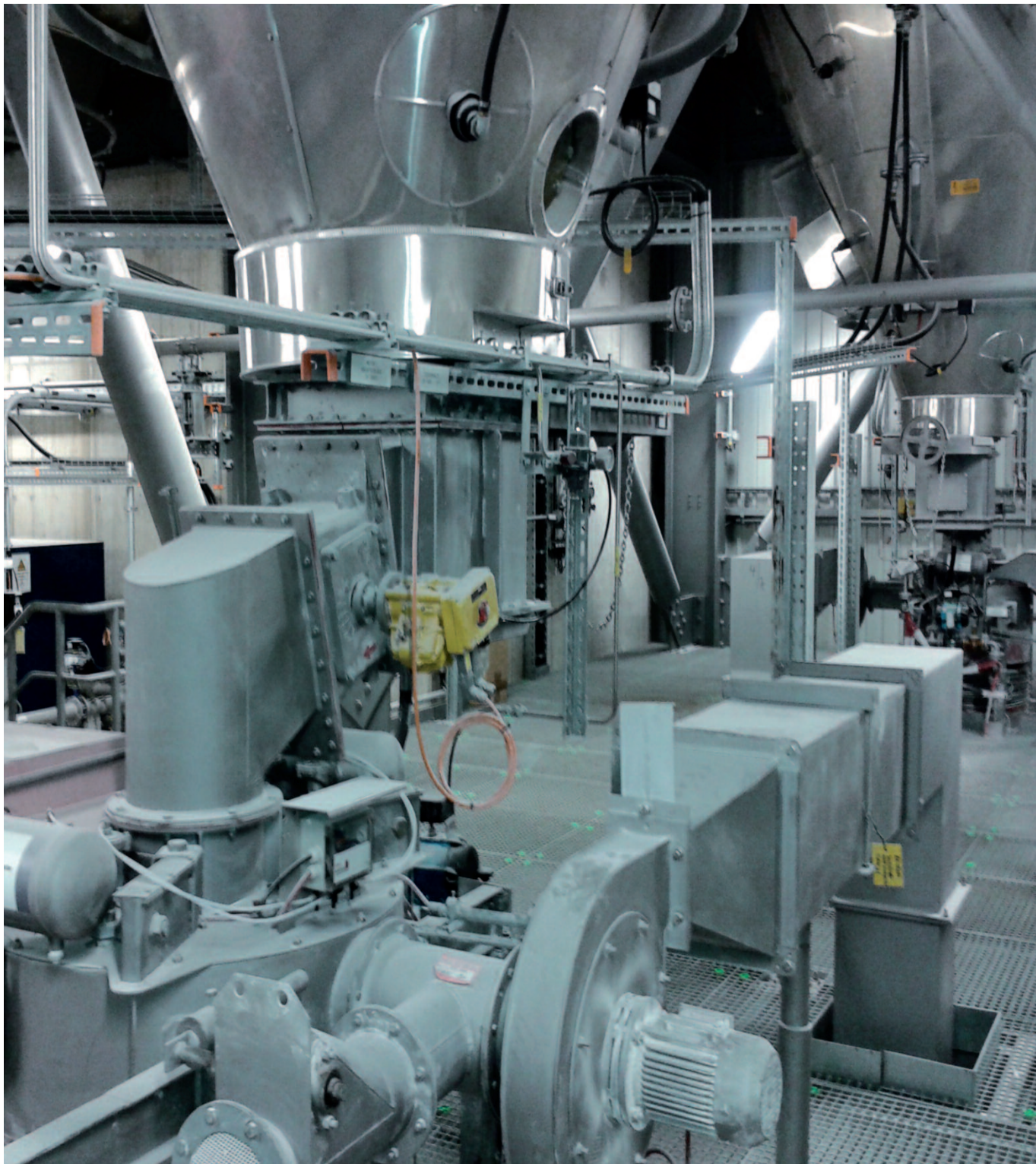
Silo discharge with loading chute for FGD product
