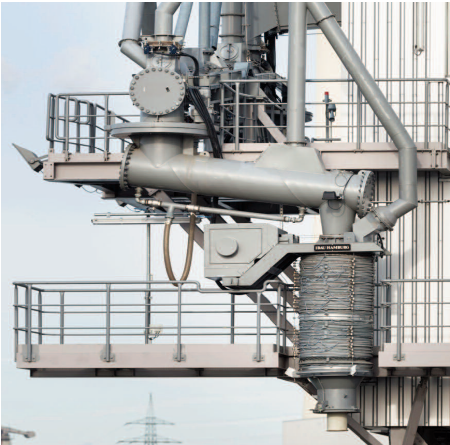
Ship loading system for dry fly ash
