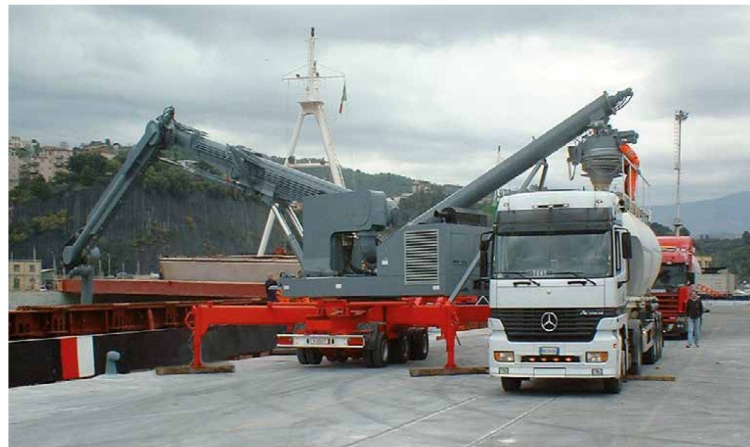
Road-mobile ship unloader for Betoncem, Port of Savona, Italy
