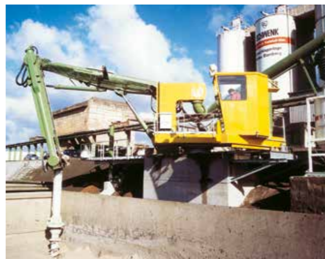
Stationary ship unloader at Bamberg Harbour, Germany
