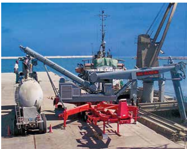
Road-mobile ship unloader in Saudi Arabia
