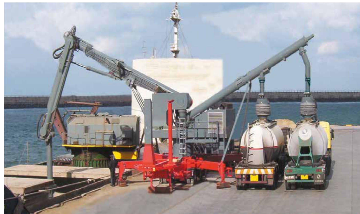
Port-mobile ship unloader for Tong Yang Cement Corporation, Korea
