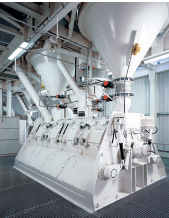
Batch-type mixer with toggle lever system
