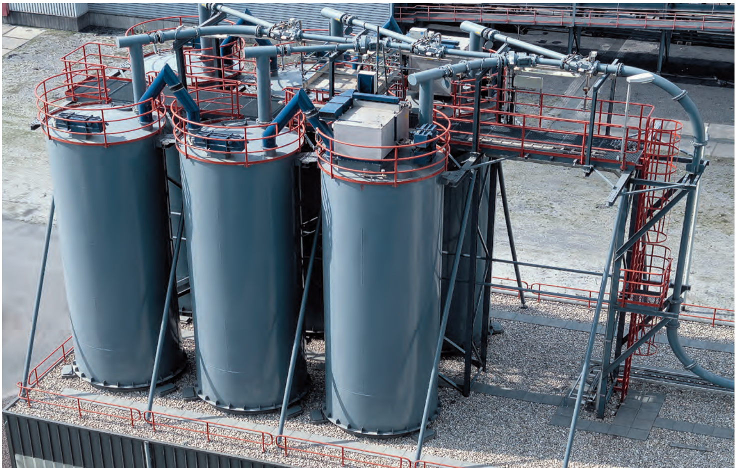
Material distribution via two-way valves into different silos
