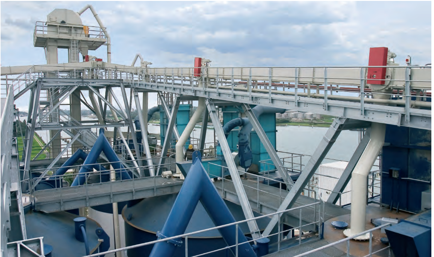
Bottom discharger for feeding different silos in a cement terminal
