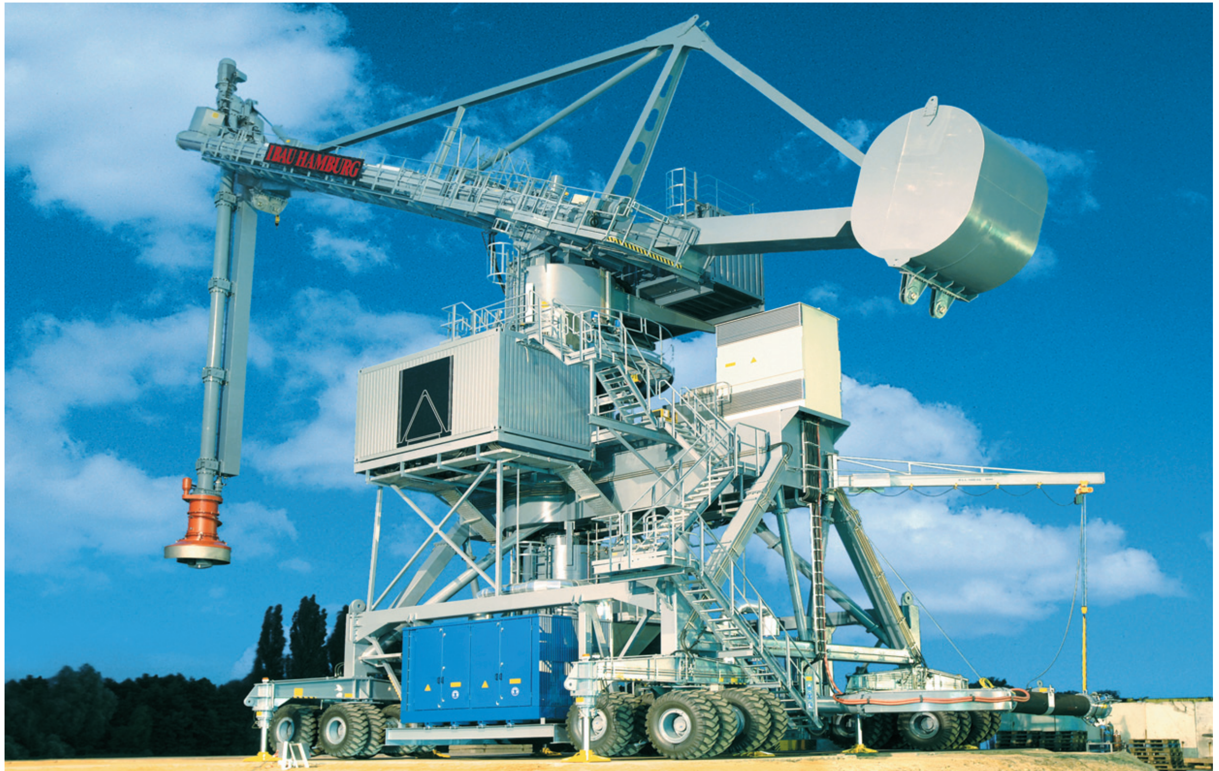
High capacity shipunloader with pneumatic conveying system
