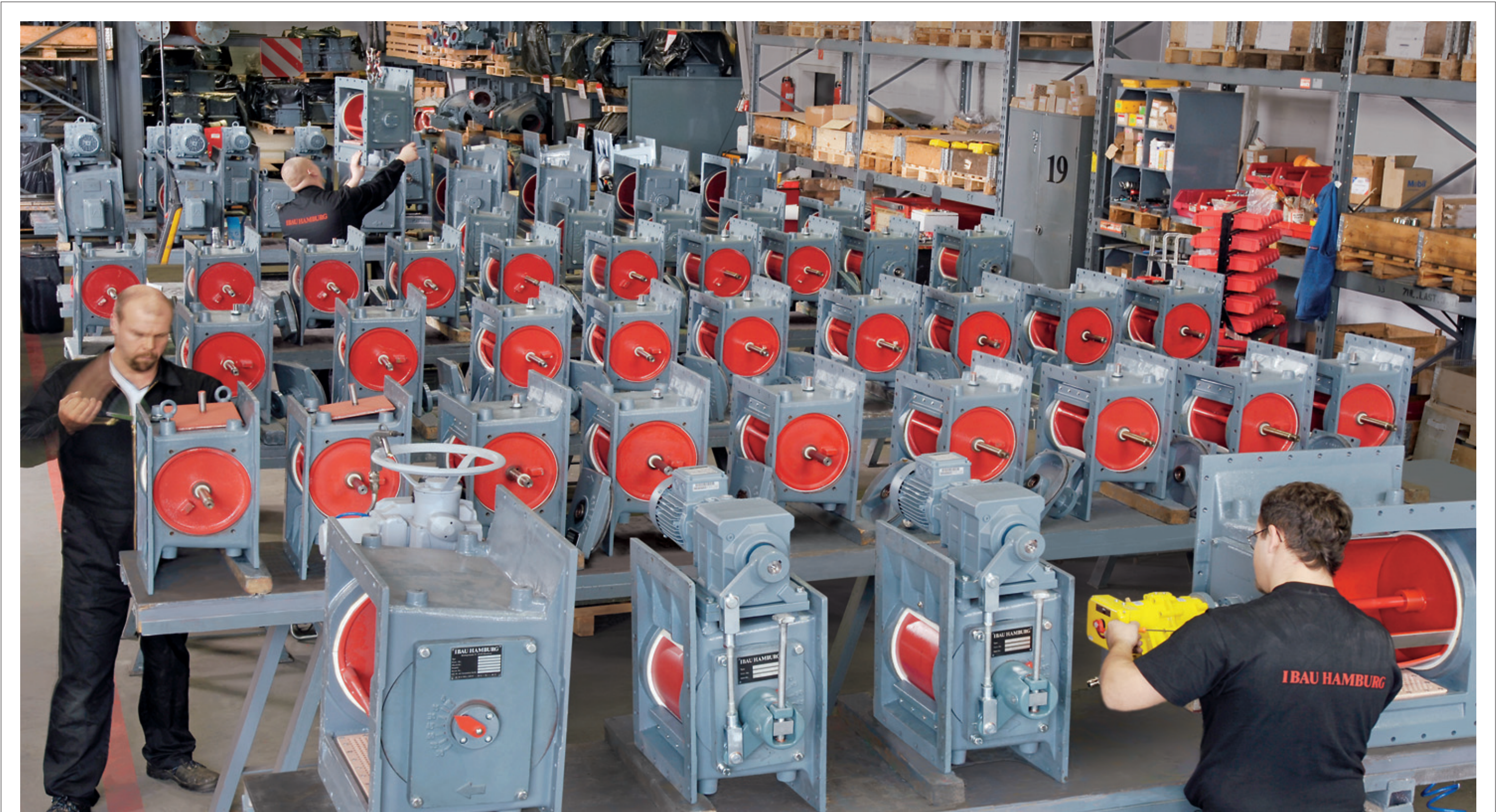
Assembly of IBAU Flow-control gates at the Hamburg-Allermöhe workshops
