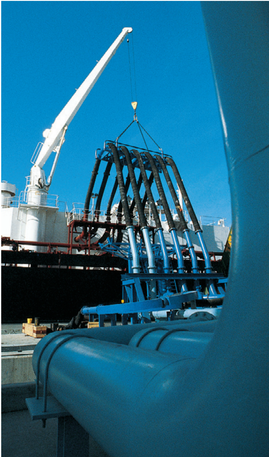
M.V. GOLIATH board crane lifting the loading pipes
