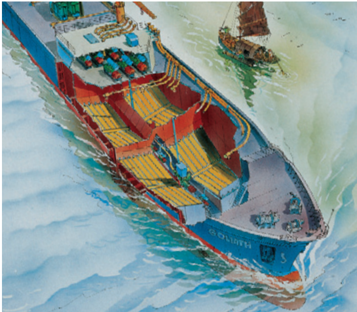
Cargo holds with aeration panels and fluidisation system with feeding of the IBAU Pump
