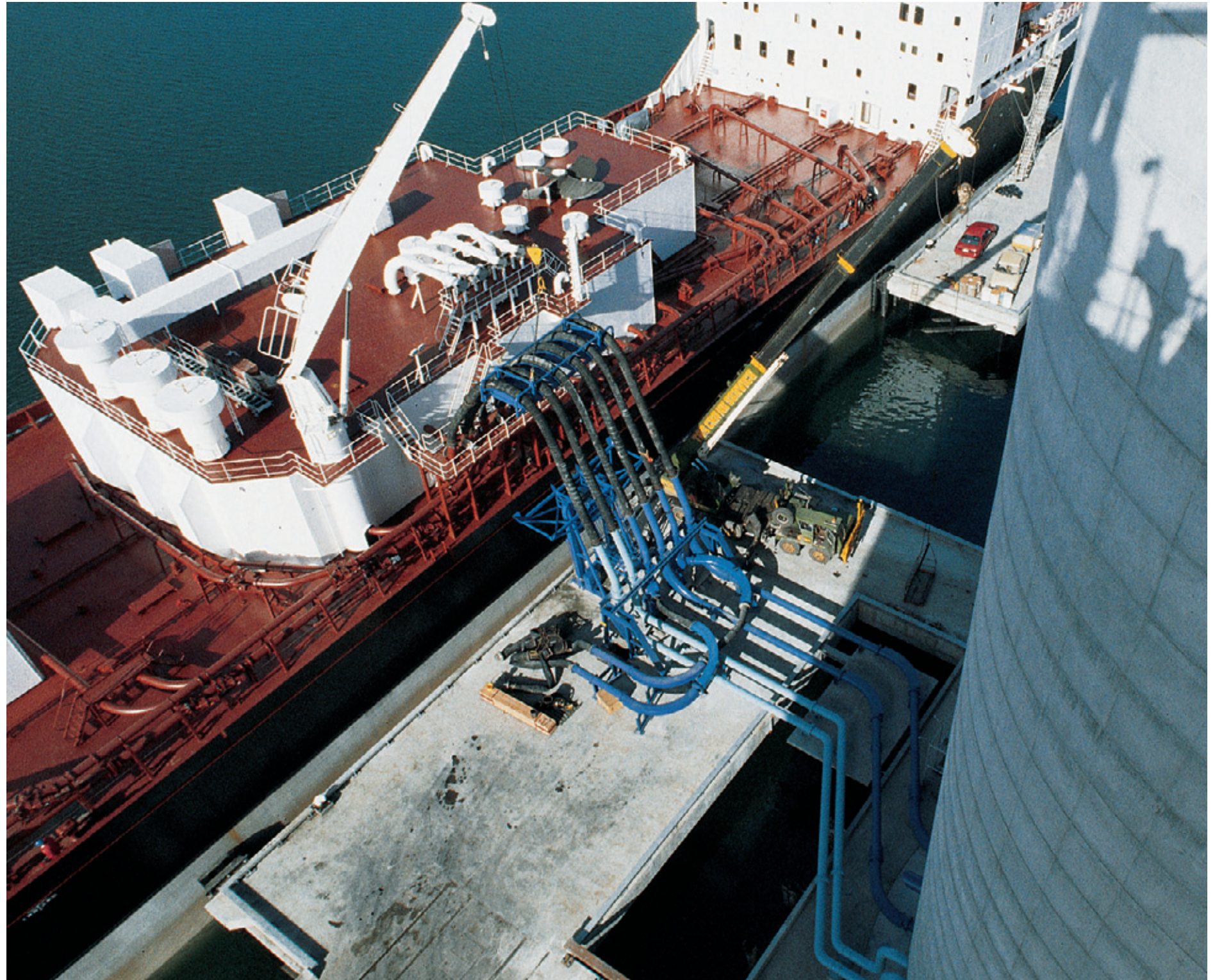
M.V. GOLIATH loading procedure for dustfree loading independent from any weather conditions
