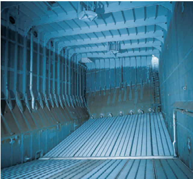
The IBAU HAMBURG Tunnel concept: Midship tunnel with IBAU Pump and aeration panels.
