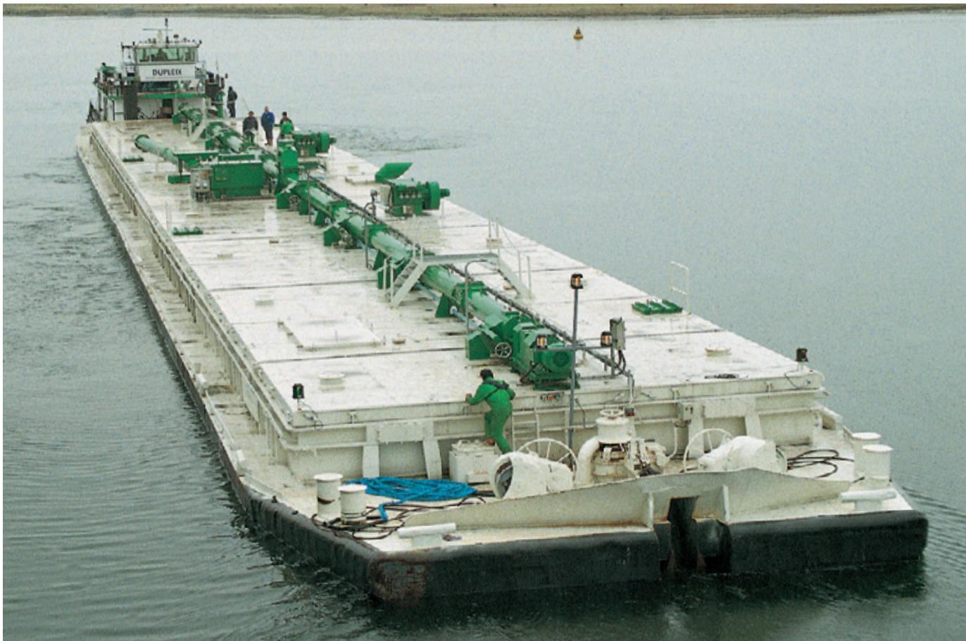
The cement barge reaching the unloading station
