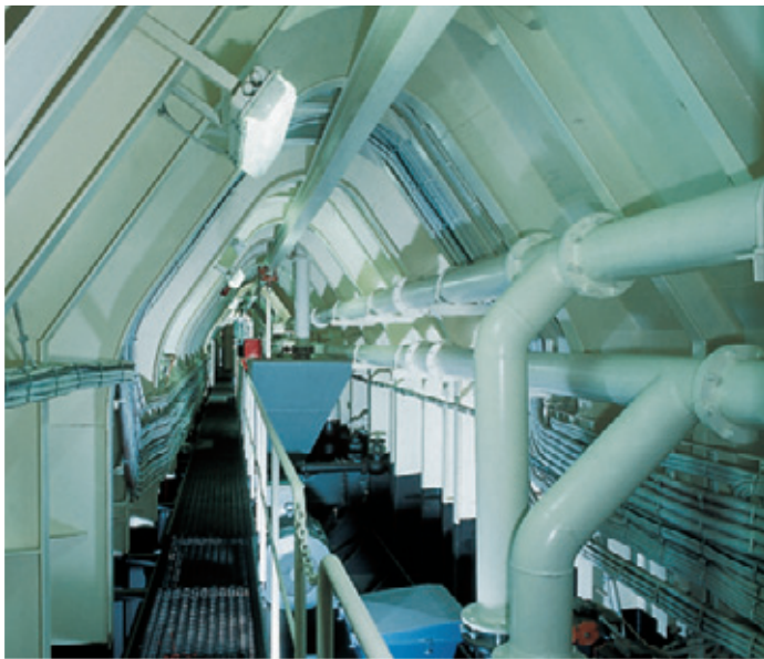
The IBAU HAMBURG Tunnel concept: Midship tunnel with IBAU Pump and aeration panels.
