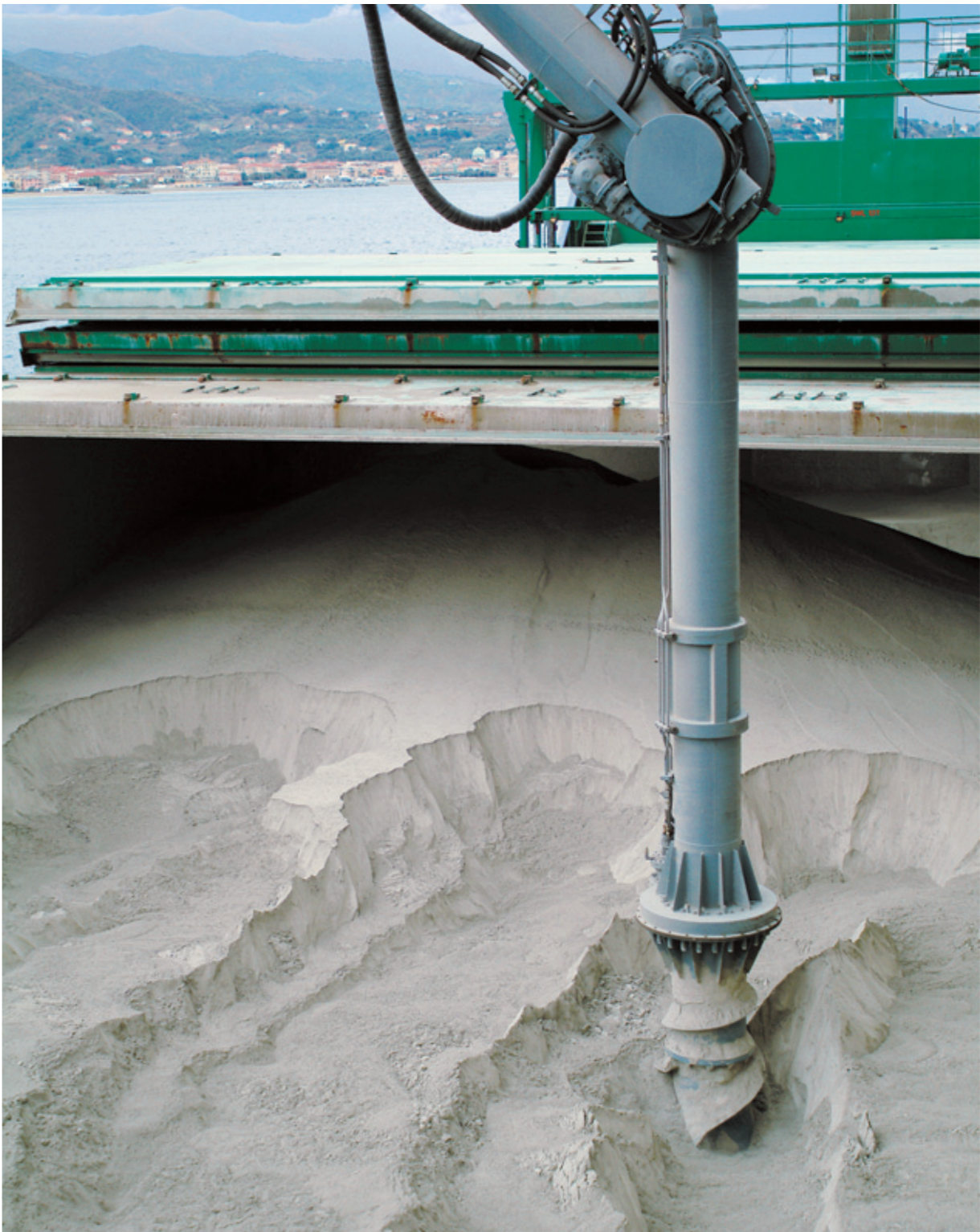
Unloading procedure, layer by layer
