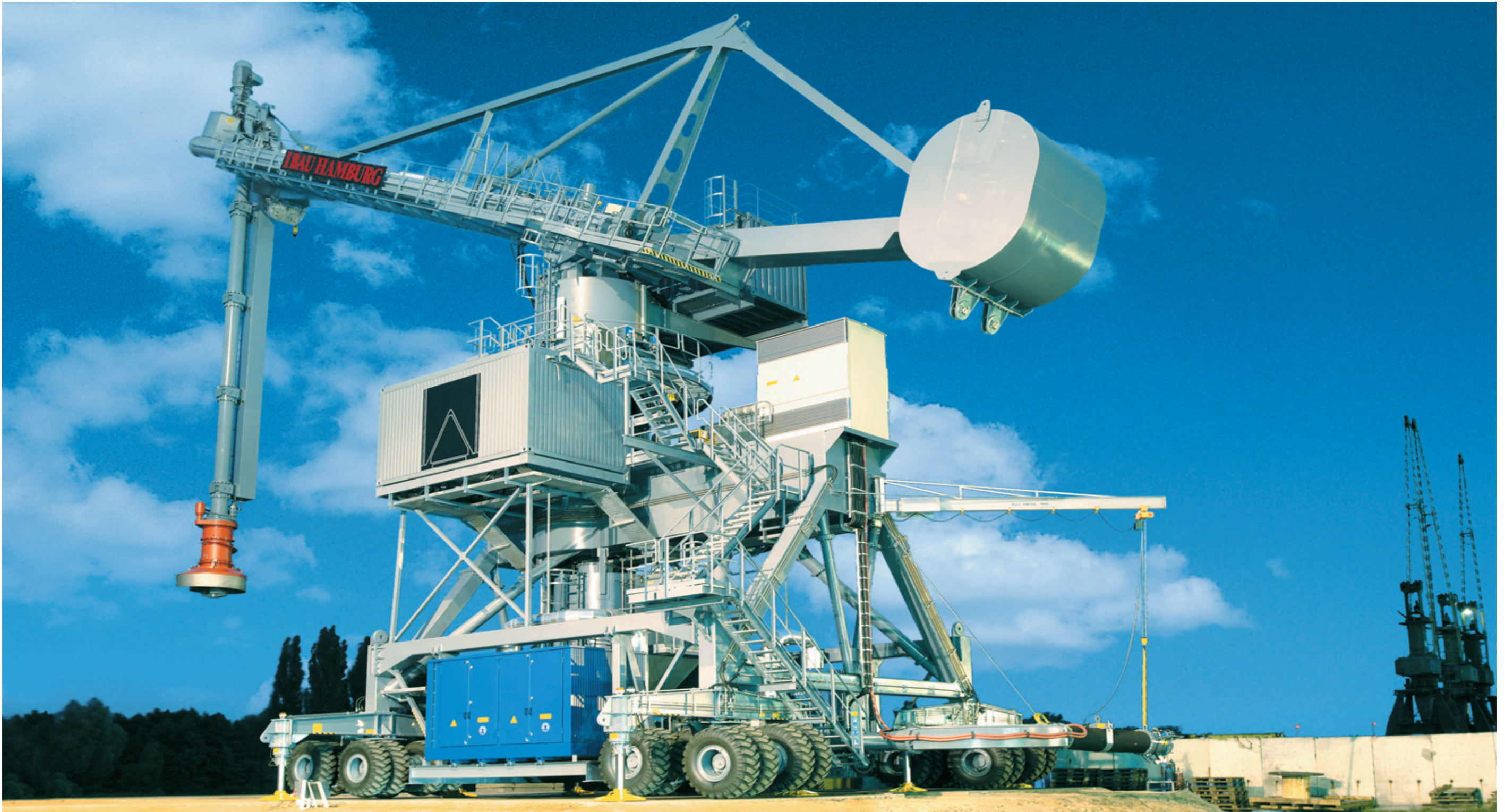
High-capacity ship unloader with on-board pneumatic equipment
