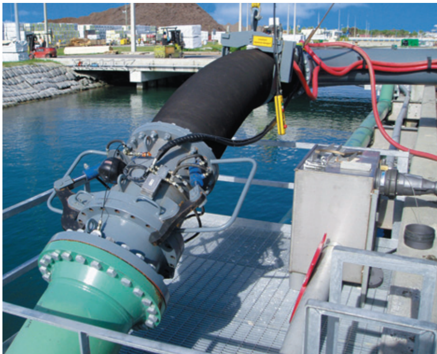
Hydraulic clamp connection to the conveying pipeline
