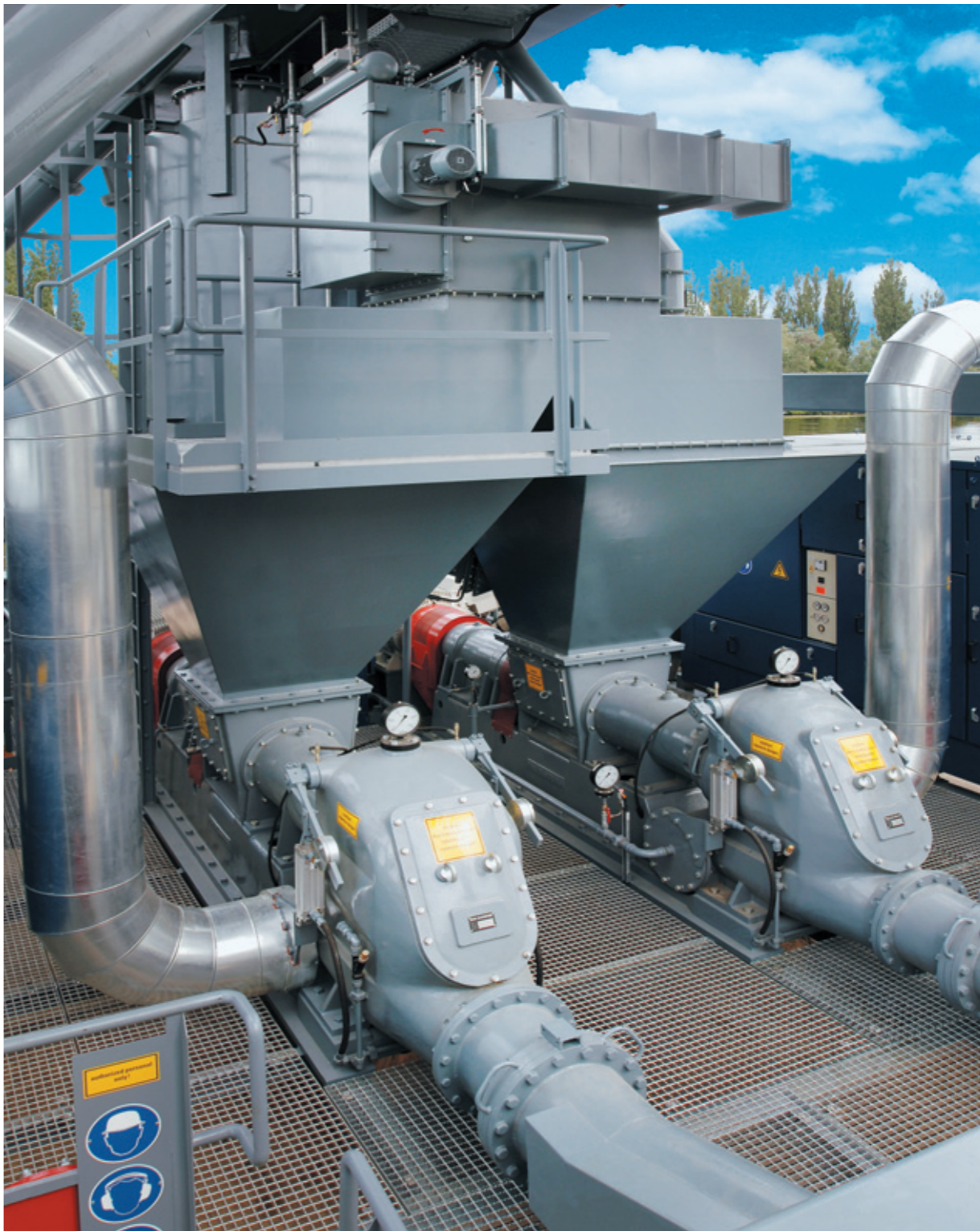
Pneumatic transport system located on the ship unloader
