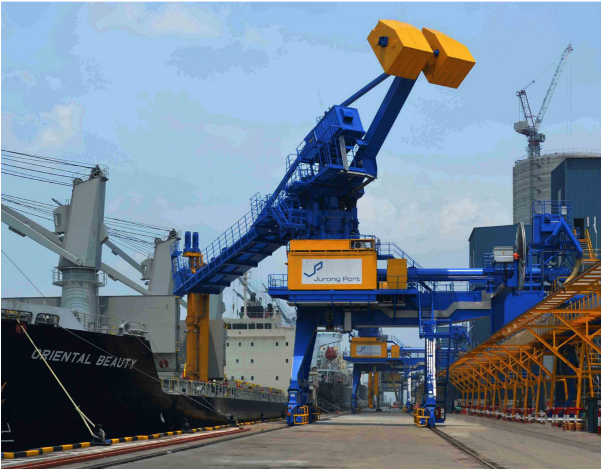
Two IBAU Ship unloaders at Jurong Port, designed for a peak capacity of 1200 t/h each, feeding a belt conveyor system.
