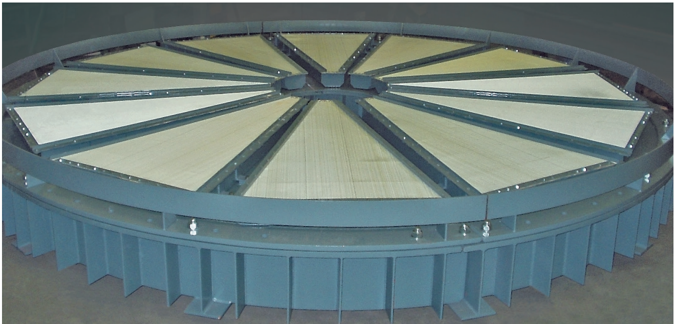
Pre-assembled silo bottom
