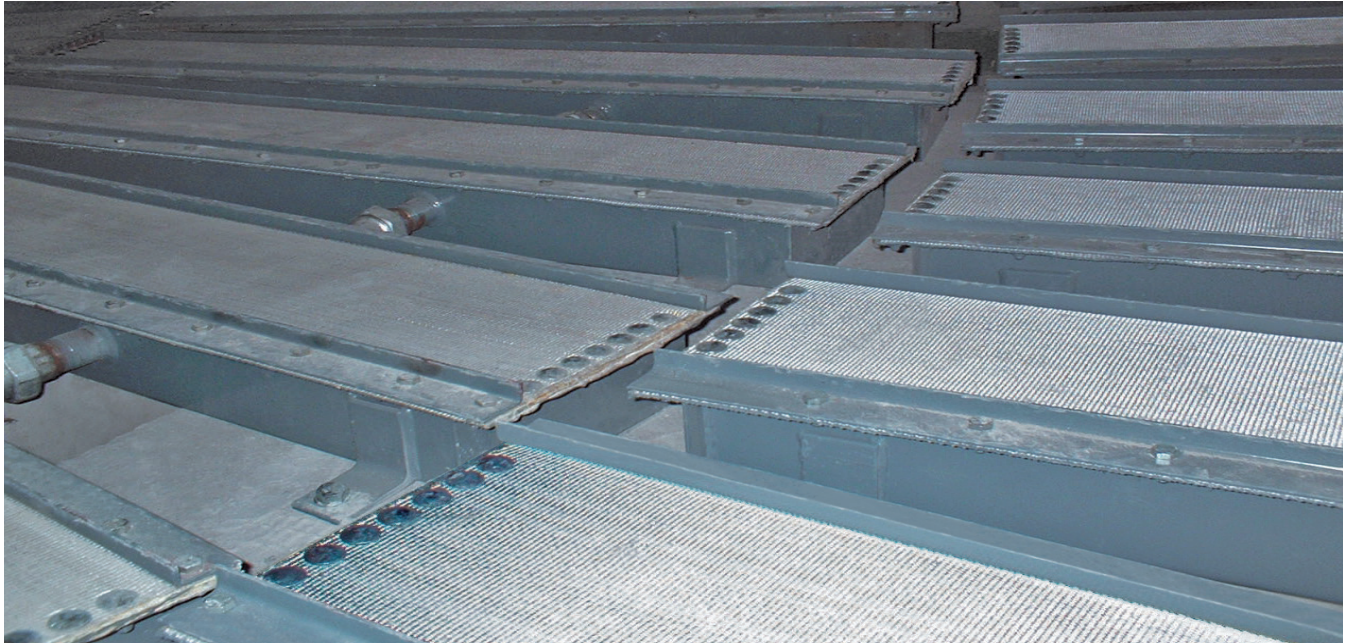
Silo aeration panels during assembly
