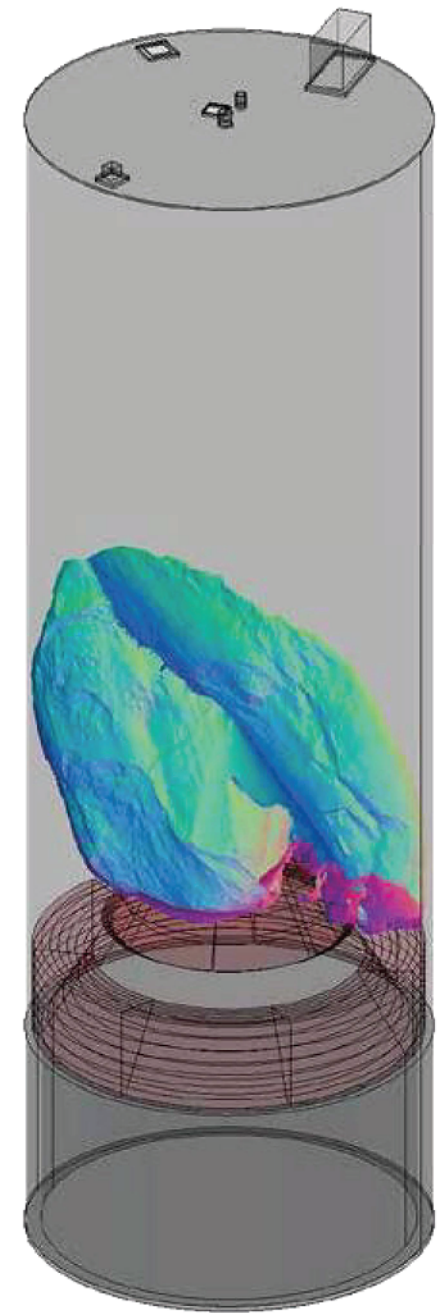
Super Imposed image of 3D Point Clouds and Silo 3D model at scale 1:1
